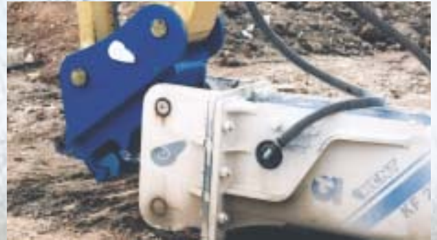
2. Articulate stick to capture rear pin ....
