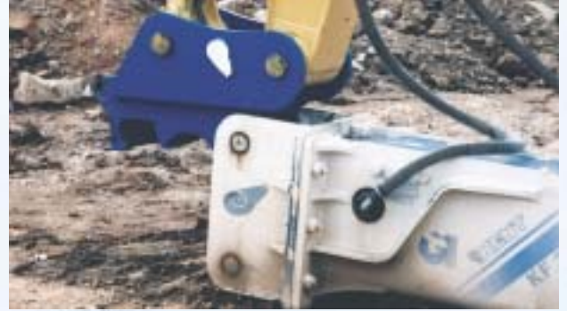
1. Position pick-up jaw over rear pin ...
