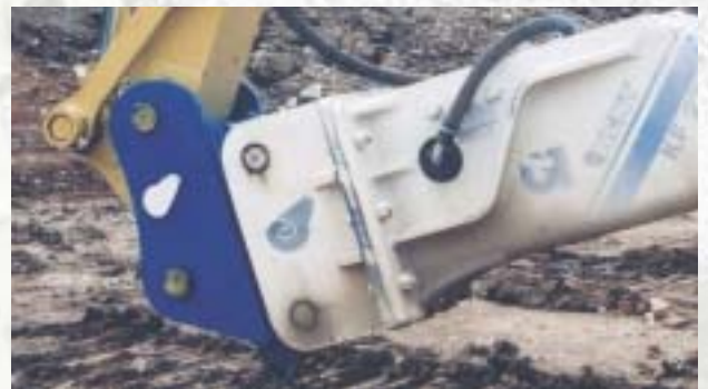
4. ... move to "full curl" position to lock and unlock.
