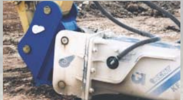
3. After rear pin engagement, extend bucket cylinder to engage front pin...
